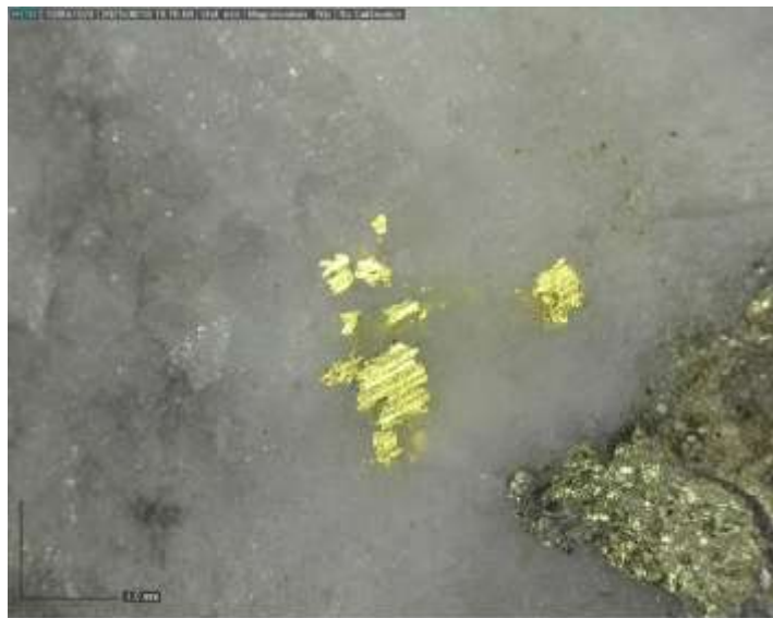
Figure 7: Visible gold from sheeted quartz veins in drillhole AX-25-746 at 243.3m.
