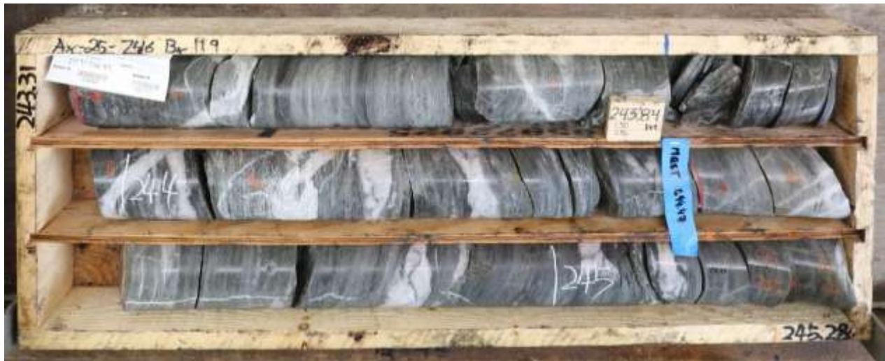
Figure 6: Mineralized interval from drillhole AX-25-746. High vein density, Bi-Sb sulphosalts and visible gold are indicative of high-grade mineralization, confirmed by assay results.
