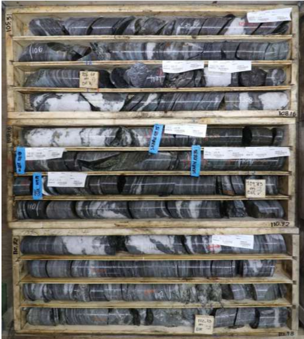
Figure 4: Mineralized zone from drillholes AX-25-690. Abundant discordant veining with coarse Bi-sulphosalts and arsenopyrite spatially associated with silicification and skarn-style mineralization (replacement mineralization of calcareous metasedimentary units).
